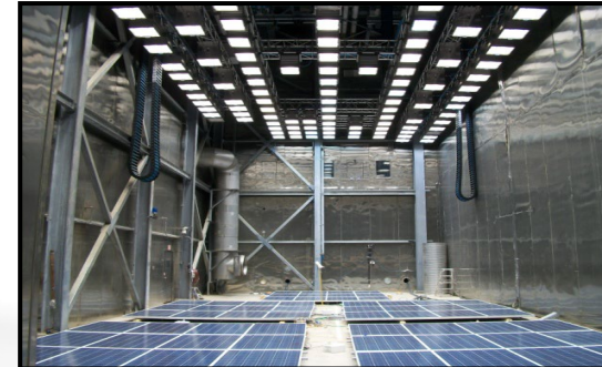
Simulated Solar for Photovoltaic Panels
