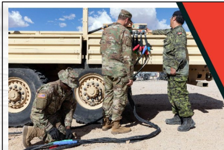
Smart Power Distribution Systems
