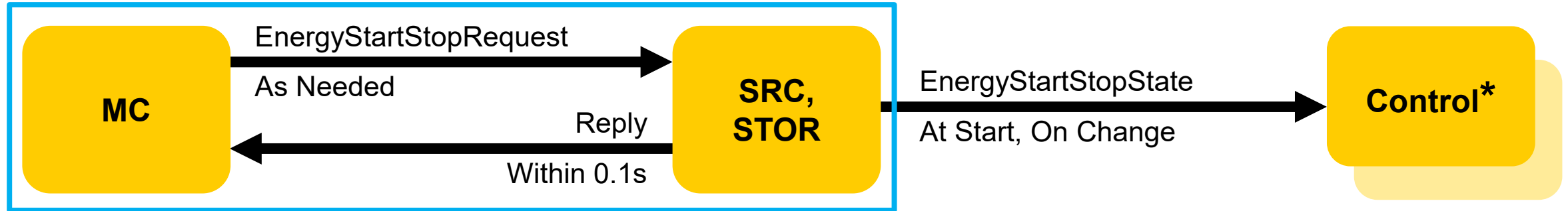
Figure B.26: Source and Storage Start / Stop Data Flow
